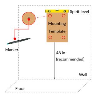
Step 2 Using a hammer drill and the appropriate drill bits for the wall material (See Preparation), drill a hole the same diameter as the anchor diameter, and at least 1-1/2" deeper than the expected embedment. Ensure that all fasteners are at least 1.5 in (38 mm) away from the edges of masonry blocks or bricks. Clean debris out the holes.
