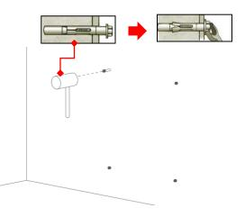
Step 4 Fasten the aPbox to the wall using the 1/4" water-tight washers (from the accessary bag), spring washers, and nuts in sequence. Use a torque wrench with an extension rod to check that the torque is 4.42 foot pounds.
