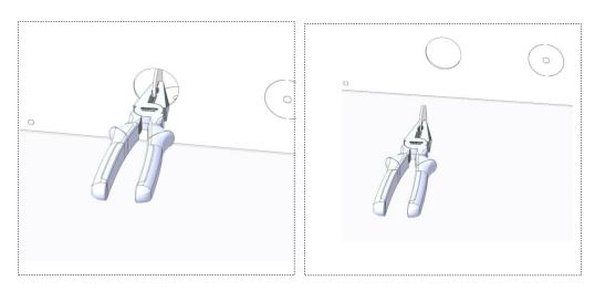
**Step 3** Dislodge the rest of the knockout. If burrs remain, remove them with a deburring tool.
