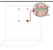
Step 3 Set the nut flush with the top of the sleeve anchor. Then, use a hammer to drive the sleeve anchor into the hole in the base material until the washer and nut are tight against the fixture. Use a 7/16" wrench to turn the nut in the counterclockwise direction, and remove the nut, spring washer, and flat washer from the sleeve anchor.
