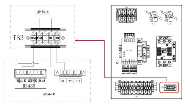
2) When one aPbox is installed on the line side of the FHP system, the communications
