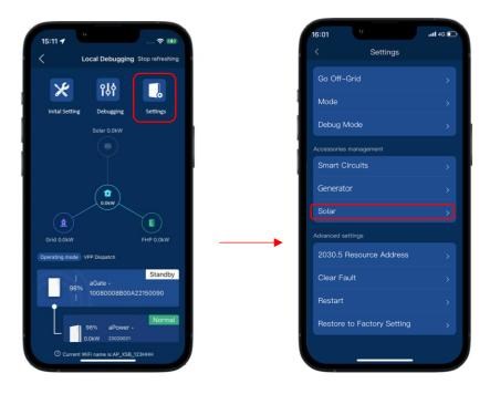
Step 3 Input the proximal solar rated power value. Enable the Remote solar access feature before setting the Remote solar, then select the appropriate access mode according to the requirements. Currently there are two kinds of access mode available, Grid-side and Load-side.
