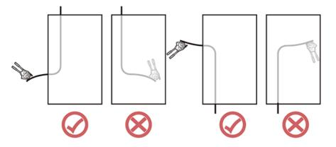
**Step 3** Insert the wires into the corresponding terminal lugs as shown in the following figure. Tighten the lugs according to Table 1 above.
