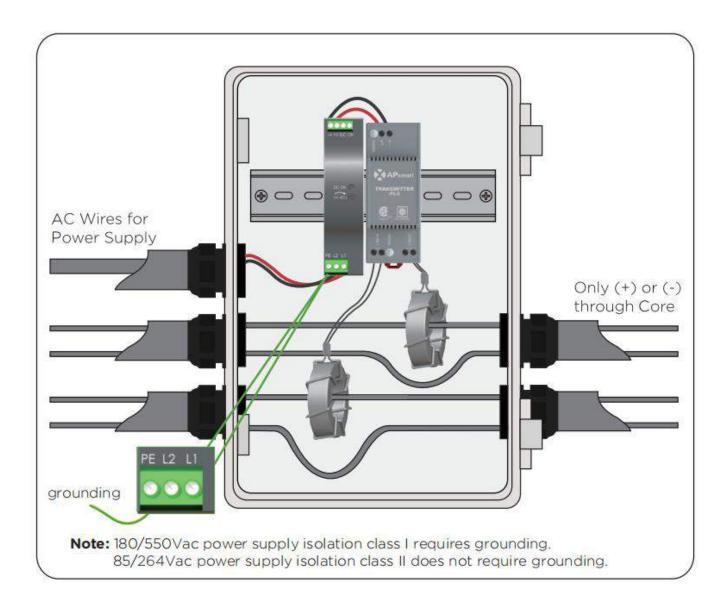
Note: Install the RSD-D before powering on the Transmitter-PLC.
