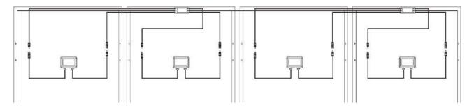
WARNING: When connecting the RSD-D to only one PV module, use INPUT1 port ONLY, then connect a DC extension cable to both terminals of INPUT2 to short the unused side, otherwise the RSD-D may be damaged.
