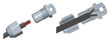
D) Insert a screwdriver into the slot on the top of the terminator to hold it in place, and tighten nut with 27 mm open-end wrench or channel lock pliers until fully tightened.
