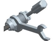
WARNING: Never unscrew the hex nut. Unscrewing the hex nut destroys the locking feature, and you must replace the terminator.
