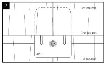
Slide flashing between 1st and 2nd course, so the top is at least 3/4" above the edge of the 3rd course and the bottom is above the edge of the 1st course. Line up pilot hole with view port.
