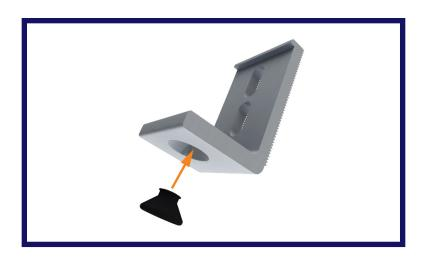
Pre-install the cone-shaped rubber SimpleSeal EPDM bushing into an EcoFasten compression bracket of your choice prior to installation by inserting the tip of the cone into the corresponding shape in the bottom of the compression bracket. The ridge around the tip of the cone will hold the bushing in place until the bracket is installed.
