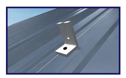
Place the compression bracket on roof surface above a supporting structural component, ensuring that the bushing sits flat against the roof surface. SimpleSeal is not designed to be installed on any ridge or corrugation of the metal roof surface.
