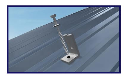
Thread the 5/16" EPDM bonded sealing washer onto the 5/16" lag bolt and insert the bolt into the top of SimpleSeal EPDM bushing.
