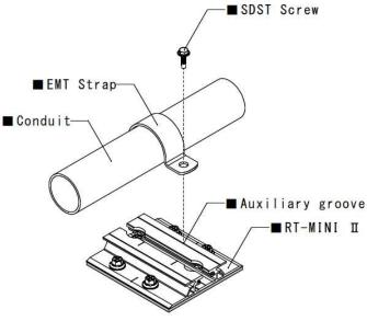
② Use the SDST screw to fix the conduit Strap. Length of SDST screw must not exceed 5/8".
