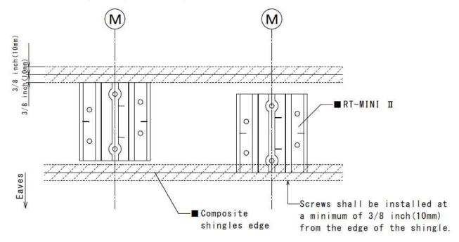
Note: The MINI II base is structurally engineered to be mounted in the above position (structural). However if used for accessories such as junction boxes or EMT with no structural value, It can then be mounted on any orientation.
