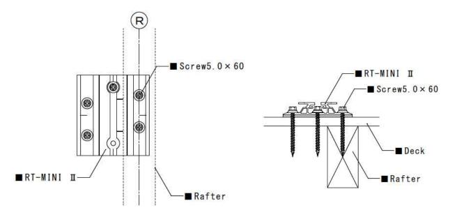
$\odot$  Deck installation: Fastened to the sheathing (Plywood or OSB) with 5ea.  $M5.0 \times 60$  mm wood screws.
