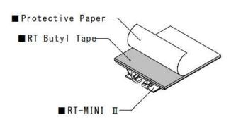
③ Place the brackets at the specified location and make sure the RT butyl attaches well to the roofing surface.
