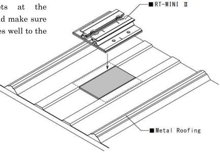
④ Set the bracket with 5 ea. (for Roof DECK), of M5.0 × 60 mm stainless wood screw using 8 mm hex socket. After completing process, make sure the brackets are securely fixed.
