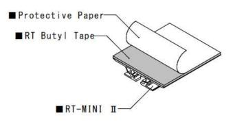
• When there are gaps in the position to install, fill them in with the additional RT butyl tape.
