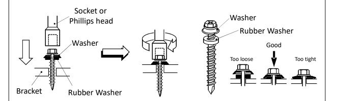
When tightening the screws please tighten all screws equally and avoid using an impact driver as it can over torque the screws or even snap off the head.
