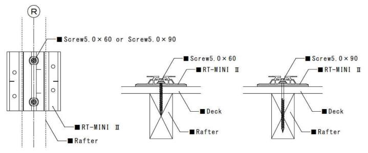
② Rafter installation (Offset): Fastened to the Rafter offset with 2ea. M5.0  $\times$  60 mm wood screws on either side and 3ea. M5.0 $\times$ 60 mm wood screws to the sheathing.
